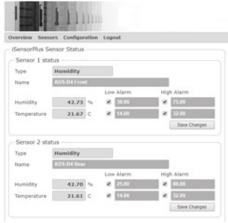
Each iSensor controller includes a fully configurable webserver to enable standalone configuration and monitoring of up to 24 sensors.
