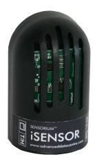
24 Temperature & Humidity sensors are included for deployment across the data centre utilising standard CAT5/6 cabling (to a maximum distance of 100m).
