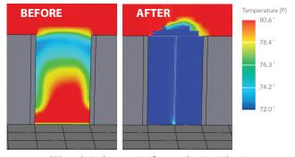
CFD analysis shows a significant reduction in hot air recirculation when aisle-end doors applied in conjunction with Rack Top Baffles at the end of the cold aisle.
