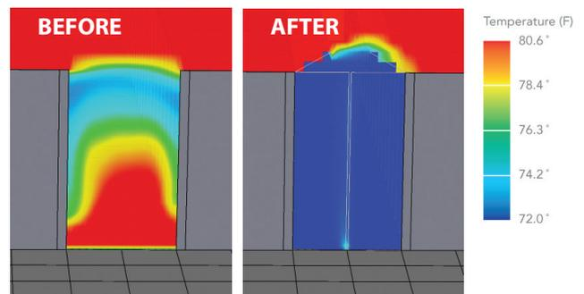
CFD analysis shows a significant reduction in hot air recirculation when aisle-end doors applied in conjunction with Rack Top Baffles at the end of the cold aisle.
