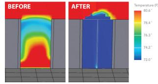
CFD analysis shows a significant reduction in hot air recirculation when Bi-Directional Doors are applied in conjunction with Rack Top Baffles at the end of the cold aisle.
