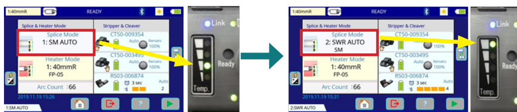
Heat temperature changes in accordance with Splice mode
