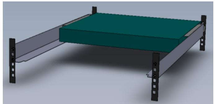
3. Before installing the chassis/extender the unit must be extended to the longest length. This is done by pulling the tabs on the inner chassis away from the extender. The cables that attach to the back of the data switch must be in place to route through the brush strips when the chassis/extender is pushed into place.
