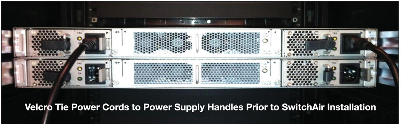
2. Before installing SwitchAir; remove the lower network switch mounting screw from each side of the rack front rails (if necessary). Save these screws to be used in the next step for mounting the SwitchAir. The network switch upper screw will remain fastened.
