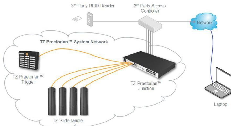
Data centre cabinets connected to the TZ Praetorian™ System are monitored by both the access controller and the TZ Praetorian™ Junction. The status of each cabinet door is indicated on the TZ Praetorian™ Trigger and each TZ SlideHandle™.
